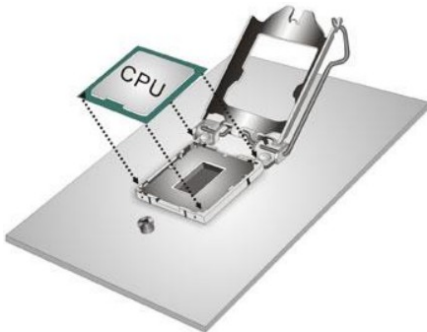
Figure 4-5: Insert The Socket LGA1200 CPU
